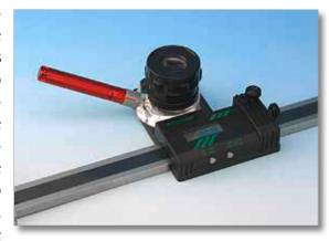
measurement can then be set by pressing the reset button. After moving the carriage to the second measuring point the result can be read off on the display. The system has an RS232 interface. This allows serial transfer of the values to the computer. An RS232-compatible interface cable with optical coupling or, as an alterna-
