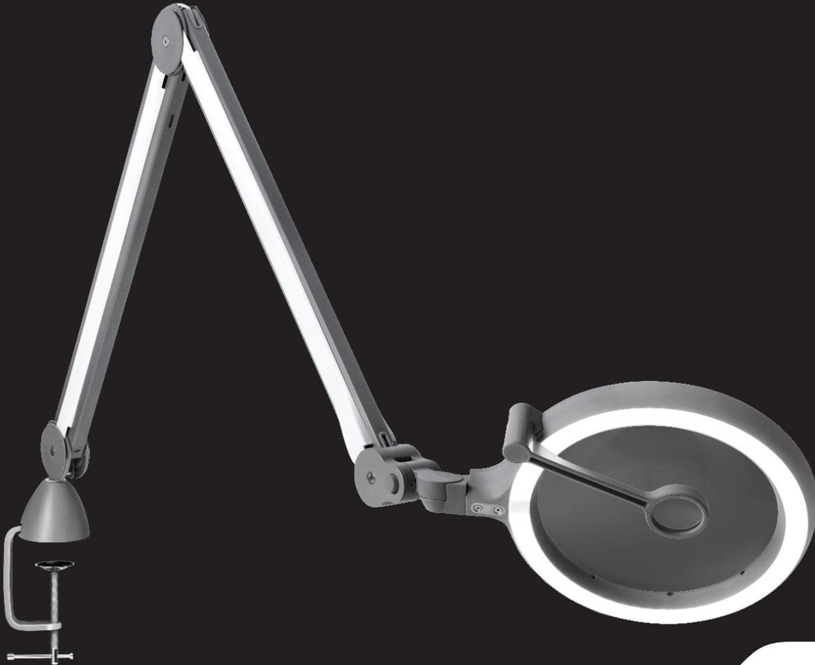
The iQ magnifier has a large and lightweight acrylic lens offering a large field of view. The magnifying head moves freely and holds any position - maximising horizontal and vertical movements. The heavy-duty internally sprung arm provides good horizontal reach and will stay in place. A 12 dioptres (4.0X) magnification lens mounted on a swing arm is also included. Lateral protections help you keep it clean. The magnifier is fitted with a removable lens protector.
