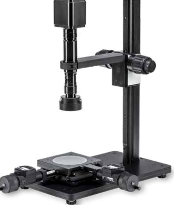
The demands on the optical system, lighting, stand and XY measurement table are a result of the inspection- or measuring job. We must take care here to use a magnification which is geared to the required inspection task.
