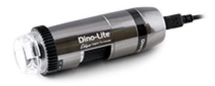
The Dino-Lite AM4917MZT is part of the Edge series, a special category within the Universal range. It offers a magnification range of 20-220x with 1.3MP and a USB 2.0 connection at 30fps. It offers superb image quality, clarity and color reproduction in a robust, compact and appealing metal housing.
