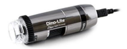
The Dino-Lite AM4917MZTL is part of the Edge<sup>\*\*\*</sup> series, a special category within the Long Working Distance (LWD) range. It offers a magnification range of 10-140x with 1.3MP and a USB 2.0 connection at 30fps. It offers superb image quality, clarity and color reproduction in a robust, compact and appealing metal housing.
