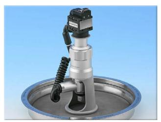
This version of our popular Cellcheck portable microscope comes with coaxial illumination making it ideal for inspecting high gloss surfaces or structures (e.g. silicone surfaces, flaws in clear finishes, chrome-plated surfaces).
