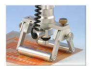
Objective Lenses with magnification factors of 2x, 4x, 6x and 10x are included as standard and can quickly be changed resulting in a magnification range from 90x to 430x on a 24" monitor. 15x, 20x and 30x objective lenses are also available as options taking magnification up to 1200x.
