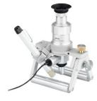
**Note:** It is essential to use the 2064-CIL-20 model in combination with the special MST tripod; otherwise the additional coaxial illumination prevents adjustment of the working distance. This applies only for the 2x lens in combination with coaxial illumination.
