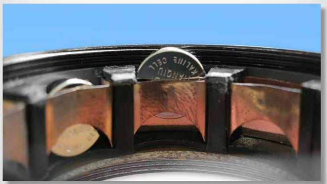
Now carefully slide the new batteries downwards into the retaining brackets. Reassemble all the parts and the battery change is finished.
